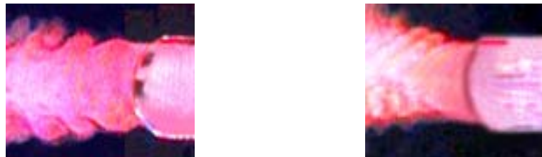
Figure 2: Smoke visualization of the classical jet under the effect of acoustic excitation at 110 Hz (left) and 250 Hz (right), flow velocity at the jet axis U_0 is equal to 5 m/s ( Re = U_0 \times d / \nu = 6667 ).
