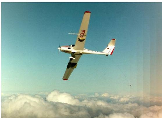
Boundary layer effects will be investigated with hot film sensor arrays or microphones and pressure tabs, alternatively, on a laminar wing glove on the G109's wing. The rectangular wing glove with an airfoil section comparable to modern glider laminar airfoils has a part with 2D flow. With this setup the influence of the turbulence level on the transition will be investigated. To gain a better insight into the receptivity process the experimental data will be compared to numerical simulations.
