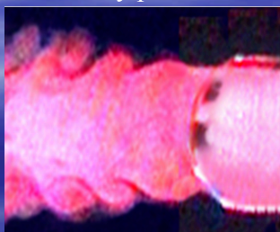
Streamwise smoke visualization pattern
