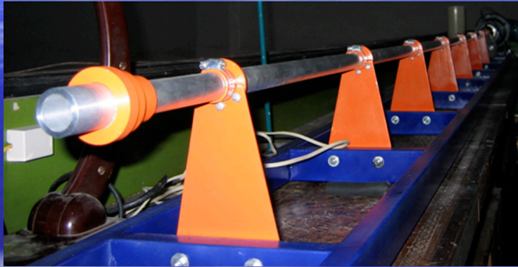
Experimental set-up with a long round channel (see left) and classical nozzle (see right)
