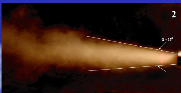
Smoke visualization of the laminar (1) and turbulent (2) jets; mean (top-right) and fluctuation (bottom-right) velocity profiles for the laminar (1) and turbulent (2) jets near the nozzle exit, flow velocity at the jet axis U_0 is equal to 5 m/s ( Re = U_0 \times d / \nu = 6667 ).
