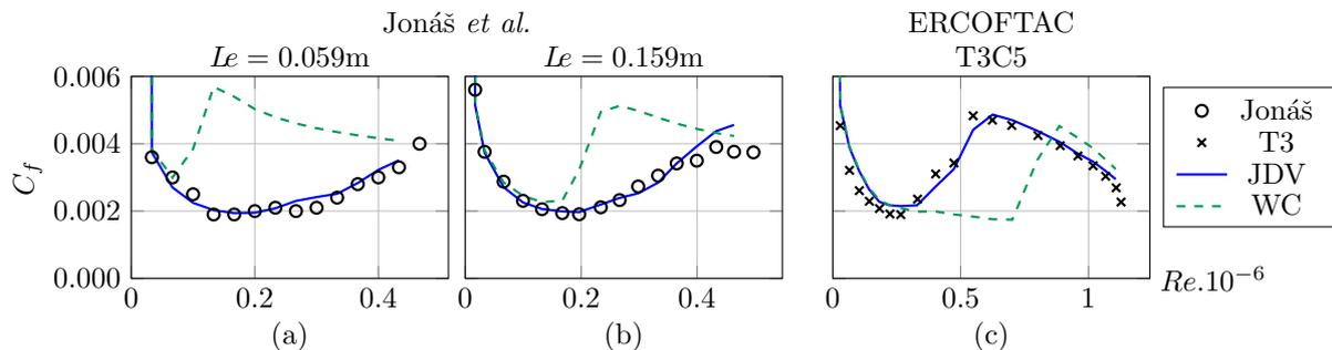
FIGURE 1. Skin friction coefficient for 2 of the 6 cases from Jonás *et al.* [7] ( $Tu = 3\%$  with different integral length scales  $Le$ ) and for the ERCOFTAC T3C5 case, with adverse pressure gradient.
