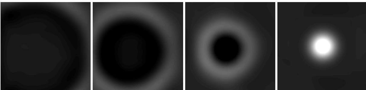
FIGURE 1. *Pressure evolution in time. The adapted boundary conditions form the desired pressure pulse.*
