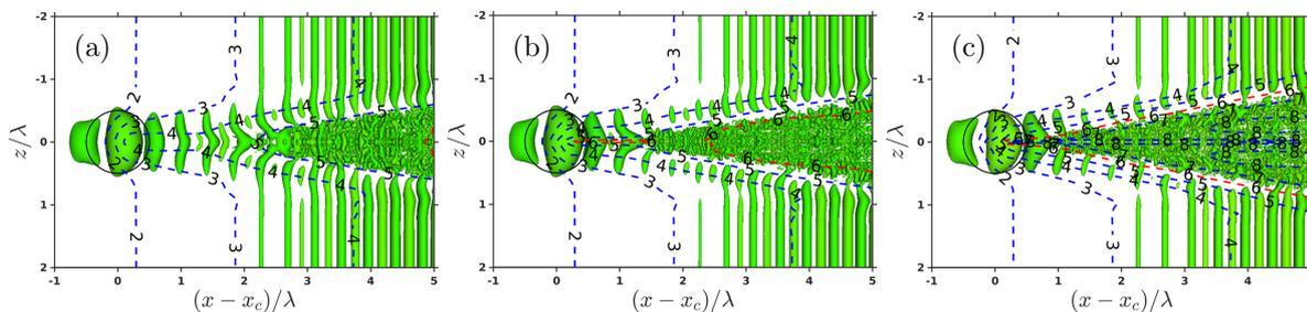
FIGURE 1. Comparison of laminar-turbulent transition onsets for different  $h$  in a large domain. The parameter  $\lambda=81\text{mm}$ . (a)  $h=1.620\text{mm}$ ; (b)  $h=1.895\text{mm}$ ; (c)  $h=2.170\text{mm}$ . The iso-surfaces are generated by pressure fields. The red dashed lines indicate the contour lines with the transition criteria  $N$ -factor 6. The solid circles indicate the indentation boundaries  $r = \lambda/2$ .
