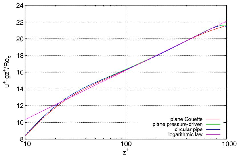
FIGURE 1. *Velocity profile after subtraction of the pressure-gradient term  $gz^+ / Re_\tau$ , compared with the logarithmic law (Luchini [1]).*
