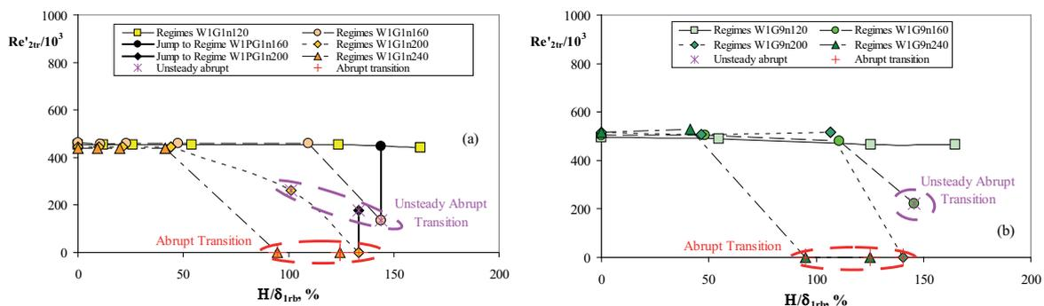
FIGURE 1. Transitional Reynolds numbers versus dimensionless roughness height obtained for various freestream speeds for elevated  $Tu$ -levels generated by grids *G1* (a) and *G9* (b) for roughness-strip width of 50 mm (case *W1*).
