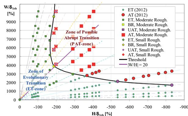
FIGURE 1. Zones of Evolutionary Transition (ET) and Possible Abrupt Transition (PAT) in plane of dimensionless values of gap depth and gap width for all cases studied in the present work. Inclined lines display constant aspect ratios  $|W/H|$  in a range from 0.5 to 100.
