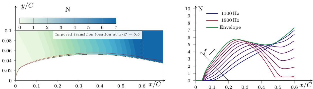
FIGURE 1.  $N$ -factor extraction on an ONERAD (symmetrical) airfoil in 2D subsonic conditions.
