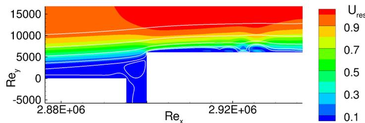
FIGURE 1. *Snapshot of unsteady flow for  $Re_h = 6000$  and sharp step, no suction.*
