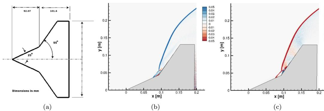
Figure 1: (a) CUBRC sharp double-cone geometry [1]. Amplitude functions of least-damped linear global mode; (b)  $\hat{u}$  and (c)  $\hat{p}$ .
