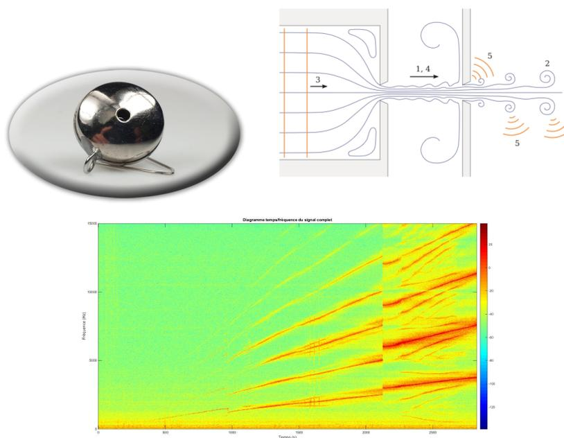
FIGURE 1. (a) : Birdcall used in this work. (b) sketch of the flow (according to [?]). (c) time-frequency diagram.
