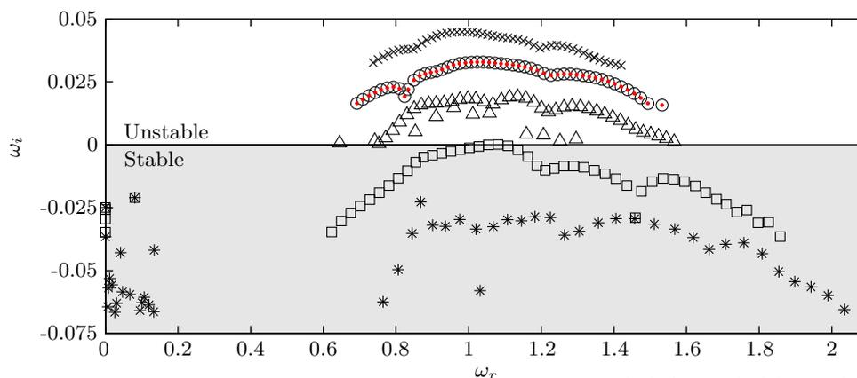
FIGURE 2. Eigenvalue spectrum for different lengths of the domain,  $460\delta_0^*$  ( $\times$ ),  $390\delta_0^*$  ( $\circ$ ),  $320\delta_0^*$  ( $\Delta$ ),  $250\delta_0^*$  ( $\square$ ),  $180\delta_0^*$  ( $*$ ), where  $\delta_0^*$  refers to the displacement thickness at the inlet.
