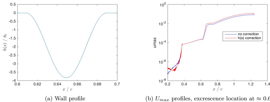
Figure 1: Dimple case  $h(x)$  profile and corresponding growth of perturbation for a frequency of 12kHz in a flat plate incompressible regime. Suction generated Tollmien-Schlichting wave around  $0.37 x/c$ .
