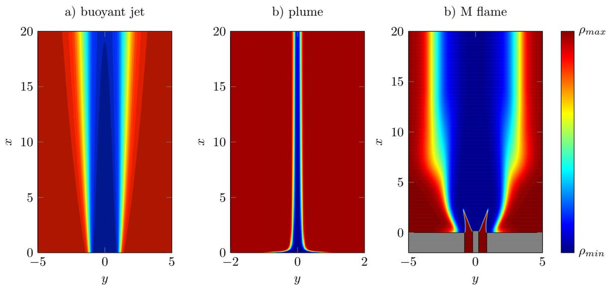
FIGURE 1. Density distributions in the meridional plane of axisymmetric base flows. Lengths are scaled with the radius of the inlet orifice. a) Jet at  $Re = 200$  and  $Ri = 10^{-4}$ ; b) plume at  $Re = 200$  and  $Ri = 10^3$ ; c) premixed M-flame at  $Re = 950$  and  $Ri = 1.6 \times 10^{-4}$ .
