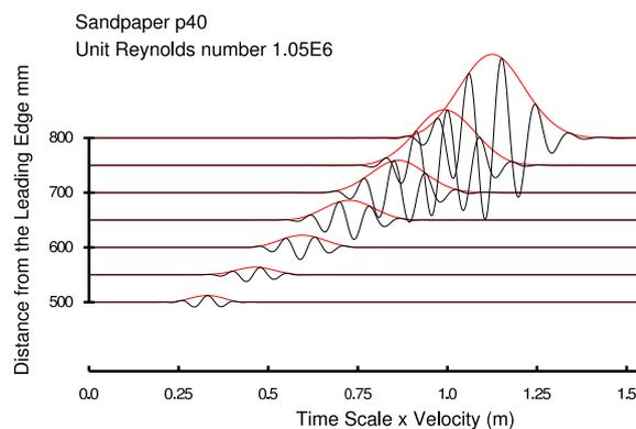
Waveform & Envelope over Roughness Panel
