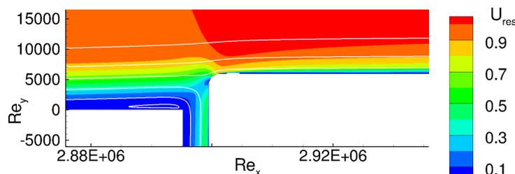
FIGURE 2. *Base flow for  $Re_h = 6000$  and rounded step, strong suction.*
