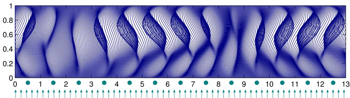
FIGURE 1. *Streaklines (in the  $x$ - $y$ -plane) of a wake past 13 cylinders. Visualized is the second least stable mode, showing a synchronization of individual units.*
