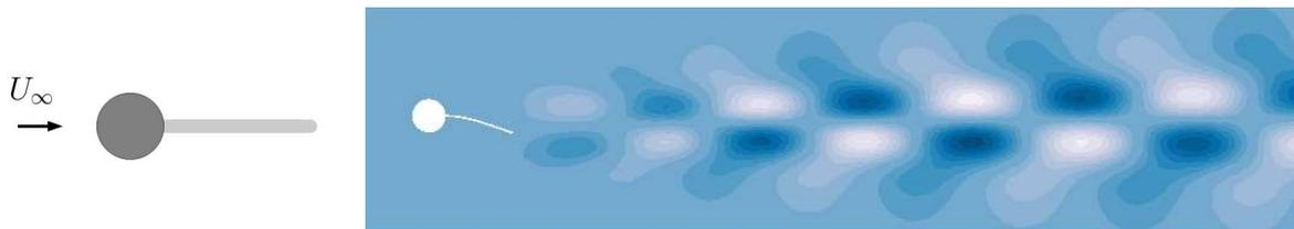
FIGURE 1. *FSI stability analysis. Left panel: sketch of the considered fluid-structure configuration. Right panel: unstable fluid-structure global mode represented by the contours of its streamwise velocity component and the corresponding shape of the structure displacement.*
