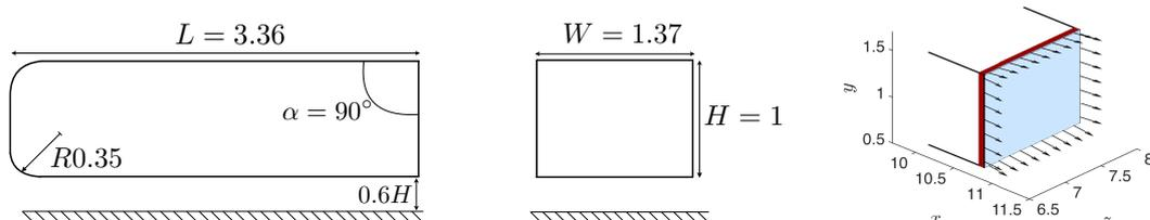
FIGURE 1. (Left) Side and rear views of simulated squareback Ahmed body. (Right) Schematic of feedback control arrangement, showing sensing (blue) and actuation (red, arrows).
