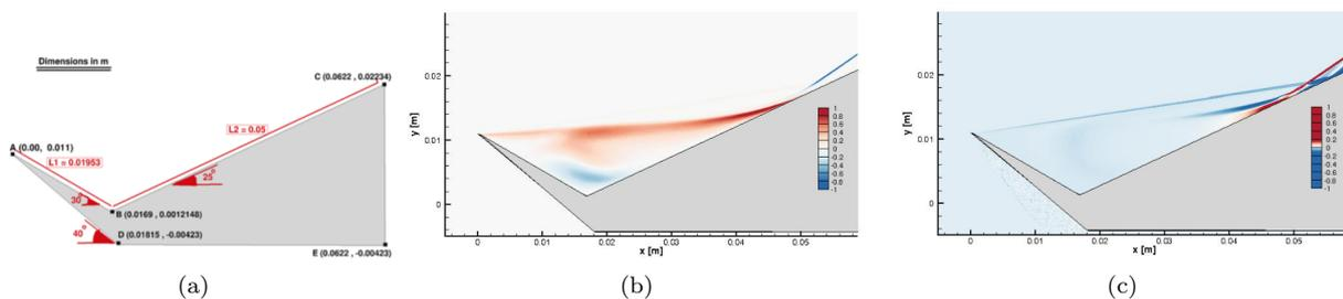
Figure 2: (a) Tick geometry. Amplitude functions of least-damped linear global mode; (b)  $\hat{u}$  and (c)  $\hat{p}$ .
