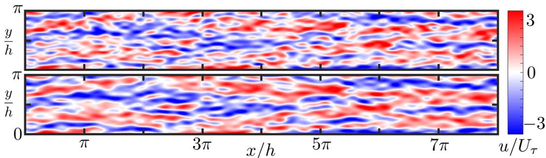
FIGURE 1. Estimation of the streamwise velocity perturbation at an instant in time at  $z^+ = 100$ . Top: True DNS velocity field. Bottom: Estimate using linear model.
