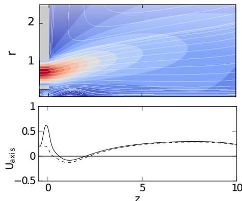
FIGURE 1. *Controlled flow field and comparison between the velocity on the axis of the uncontrolled (dashed) and controlled system.*
