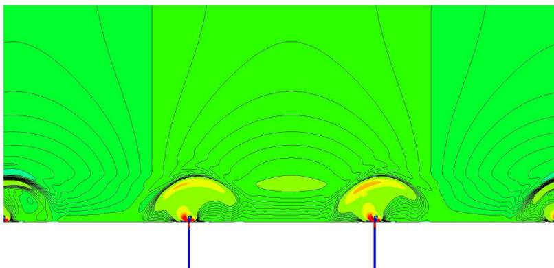
FIGURE 1. *interaction of a temporally growing TS-wave (contour-lines) with acoustic perturbations (color-coded wall-normal velocity) emitted from three suction-slots.*
