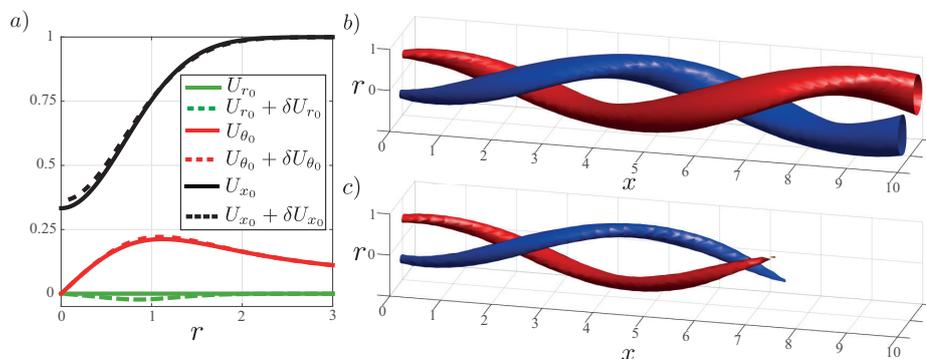
FIGURE 1. (a) Velocity components of the uncontrolled inlet condition (solid lines), which correspond to a Batchelor vortex profile, and inlet condition perturbed by the application of the control (dashed lines). Isosurfaces of the maximum axial vorticity of the corresponding global spatial mode are shown in (b) for the uncontrolled case and in (c) for the controlled case.
