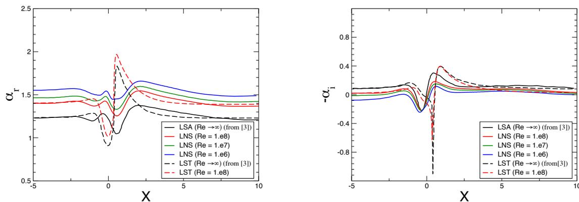
FIGURE 1. Wavenumber  $\alpha_r$  (left) and growth rate  $-\alpha_i$  (right) of a TS wave at frequency  $\omega = 3.0$  for a hump with height  $h=2.0$  and width  $d=0.5$  located at  $X = 0.0$  on a flat plate.
