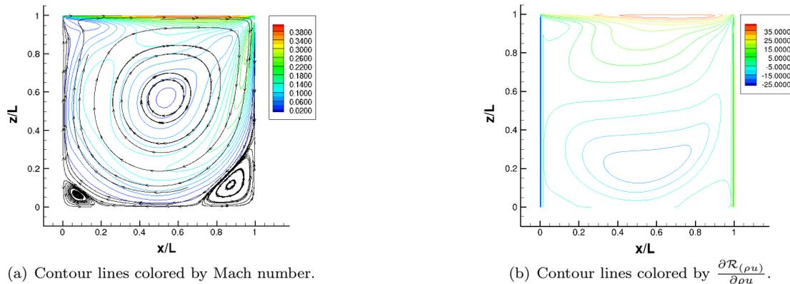
FIGURE 1. *Lid-driven cavity flow at  $Mach_\infty = .5$  and  $Re_\infty = 900$ .*
