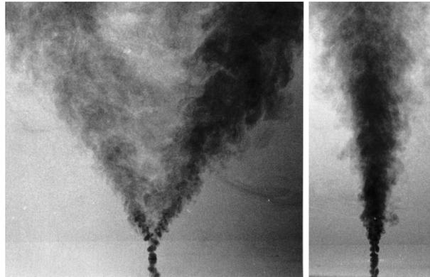
FIGURE 1. *Example of bifurcating jet ( $r_f = 2$ ) in water at  $Re \approx 20000$ , published in [1] from experiments carried by Reynolds in 1984: (left) bifurcating plane view, (right) side plane view.*
