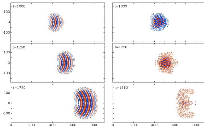
Figure 2. Evolution of a TS wavepacket at three instances of time,  $t = 1000, 1250, 1750$ , without control (left column) and with control (right column). The iso-contours of the streamwise component are shown in the  $xz$ -plane at  $y \approx 1.9$ ; red isolines indicate positive velocity, while the negative one is indicated with blue. All the plots are characterized by the same isocontour range  $[-1.03, 1.03]$ .
