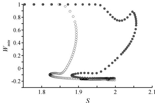
Figure 1: Minimum streamwise flow velocity in the pipe as a function of the swirl number, without control (open symbols) and with control (filled symbols).
