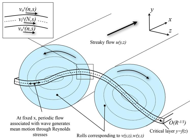
Figure 1: Sketch of critical layer intersecting rolls. The location of the critical layer varies with  $z$  where the Reynolds stresses associated with wave trapped in the critical layer generate a mean motion leading to jumps in the roll normal shear and pressure across critical layer with all other components of shear and velocity continuous.
