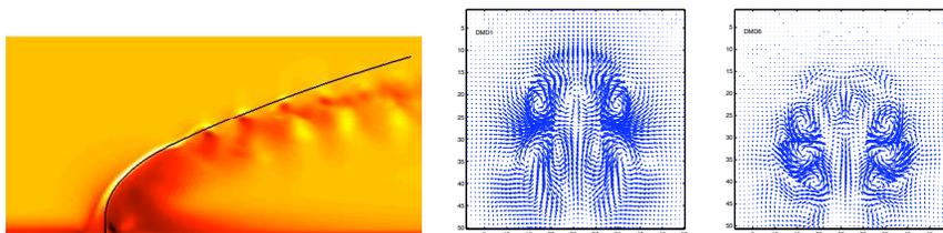
Figure 1: Spatial analysis of a jet in crossflow. (a) Snapshot from a direct numerical simulation of a jet in crossflow, including (in black) the streamline starting at the jet exit and defined by the mean velocity profile. (b) Most dominant spatial dynamic/Koopman mode. (c) Representative higher dynamic/Koopman mode.
