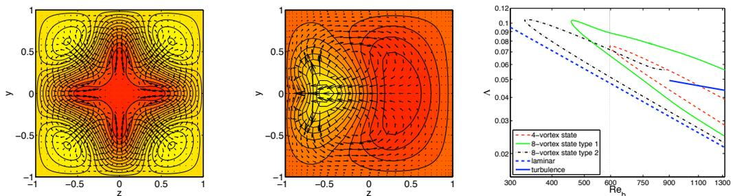
Figure 1: Two structures in square duct flow, averaged over the streamwise direction. The arrows represent the cross-stream velocity and the contour levels the streamwise velocity. Left: an 8-vortex TWS (named type 1),<sup>2</sup> similar to observations in turbulence. Middle: the edge state, expected to have connections to the transitional regime. Right: The skinfriction  $\lambda$  as a function of the bulk Reynolds number  $Re_b$ .<sup>2,3</sup>
