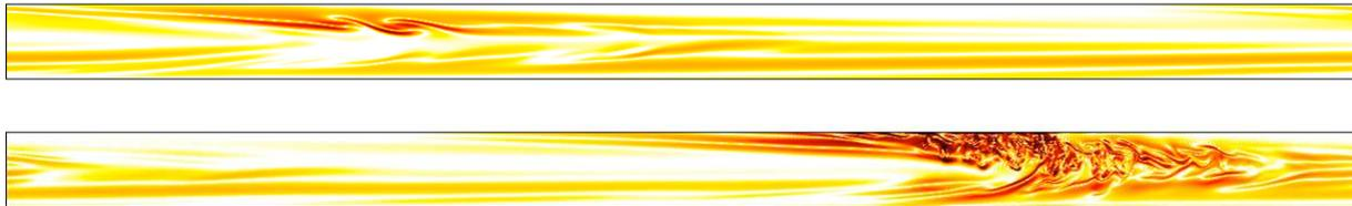
Figure 1: Direct numerical simulation of the formation of a slug in pipe flow at  $Re = 4500$ , starting from the instability of the corresponding edge state. Logarithmic iso-contours of the azimuthal vorticity perturbation in a meridian plane. The mean flow is from left to right.
