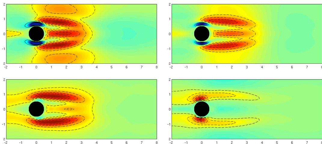
Figure 1. Sensitivity w.r.t. amplitude (top) and frequency (bottom). In each row; (left) limit cycle, (right) linear stability analysis of stationary baseflow. Negative values (dashed), positive values (solid).
