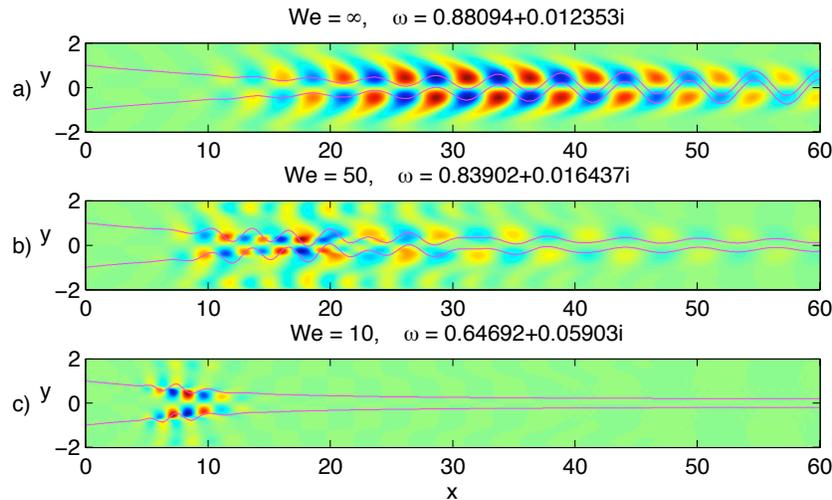
**Figure 2:** Real part of the streamwise disturbance velocity for the most unstable global mode of the same example wake as in figure 1, with increasing surface tension (decreasing  $We$ ) from top to bottom. The eigenvalue  $\omega$  is given above each figure. The disturbed position of the interface is illustrated by the magenta line, but its oscillation amplitude is only determined up to a constant.
