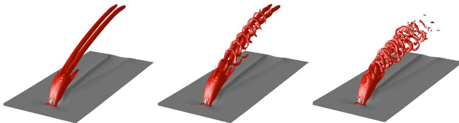
Figure 1: A jet in crossflow: The unstable steady solution (left figure) is modified by finite-amplitude disturbances (center figure) and eventually develops into a fully unsteady and nonlinear flow (right figure).
