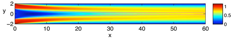
**Figure 1:** Streamwise base flow velocity for an example wake ( $Re = 316$ ,  $h = 1$ ,  $\Lambda^{-1} = -1.32$ ). The position of the interface between the fluids is given by the magenta line.
