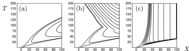
Figure 1: Contours of wave-amplitude,  $A(X, T)$ . (a) b.c.  $A \rightarrow 0$  as  $X \rightarrow \infty$ : global stability. (b) b.c.  $A(100, T) = 0$ : global instability. (c) With stabilizing nonlinearity.
