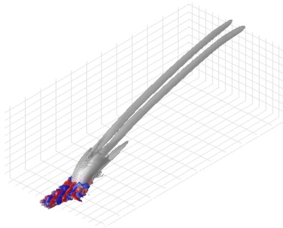
Figure 1: The  $\lambda_2$  vorticity criterion for the base flow (grey), is shown together with the wall-normal velocity of the leading adjoint eigenmode (red and blue isocontours correspond to positive and negative velocities respectively).
