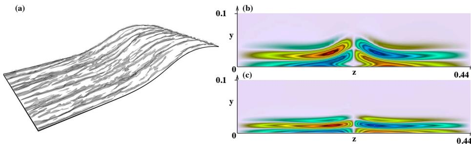
Figure 1: (a) Skeleton of instantaneous low-speed streak structure along the curved lower wall. Streamwise vorticity in the  $(y, z)$  plane of instability mode at (b) upper wall, (c) lower wall.
