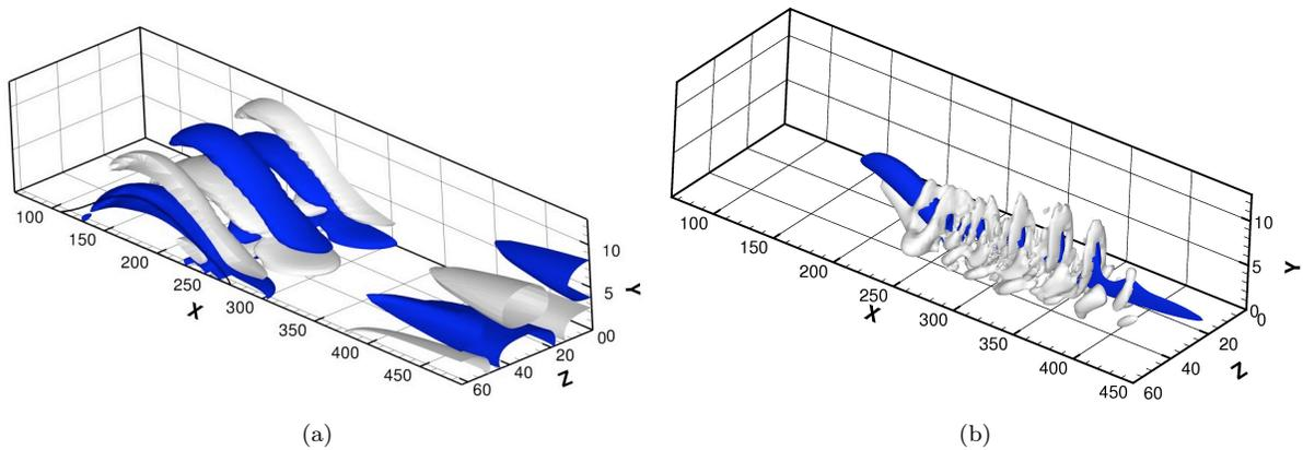
Figure 1: Iso-surfaces of negative and positive (white and blue surfaces, respectively) spanwise vorticity for the less stable steady mode obtained by global eigenvalue analysis (a); iso-surfaces of the vortical structures (white surfaces) and of the negative streamwise perturbation (blue ones) obtained by DNS at  $t = 10000$ .
