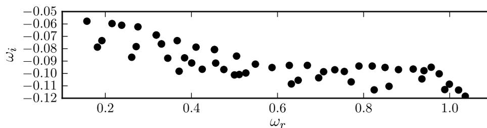
Eigenvalue spectrum of an isothermal jet at  $Ma = 0.9$  and  $Re = 100$ .
