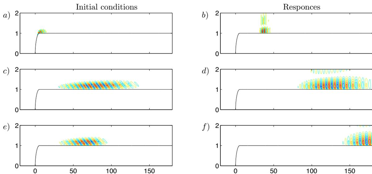
Figure 1: Optimal initial conditions and the corresponding responses. Optimisation times:  $t = 60$  a),b), 120 c),d) and 250 e),f) respectively. In all figures the streamwise velocity is shown while the spatial dimensions are scaled with the half thickness of the plate.
