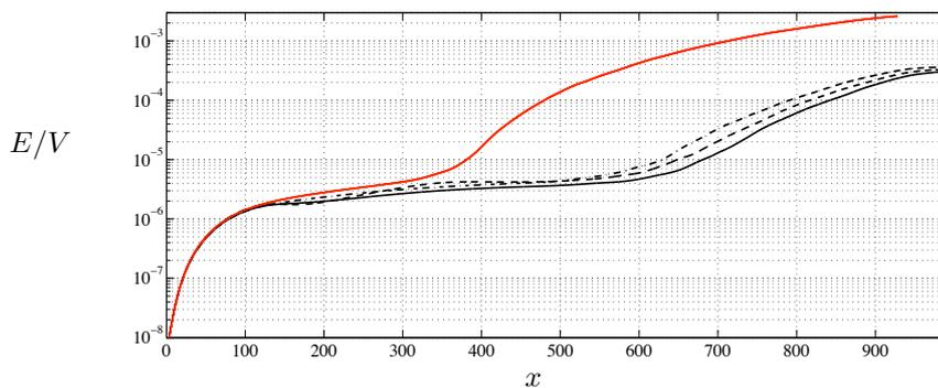
Figure 1: Energy density evolution as function of the streamwise coordinate, uncontrolled case (red) vs controlled cases (black)
