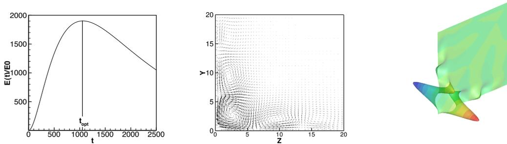
Figure 2: Left: Energy curve.  $Re_{\delta^*} = 1000$ . Middle: Optimal perturbation at  $t = 0$ . The arrows indicate  $(v, w)$  fields. Right: Optimal perturbation at  $t = t_{opt}$ . Contours represent the most amplified streamwise velocity perturbation at  $t = t_{opt}$ .
