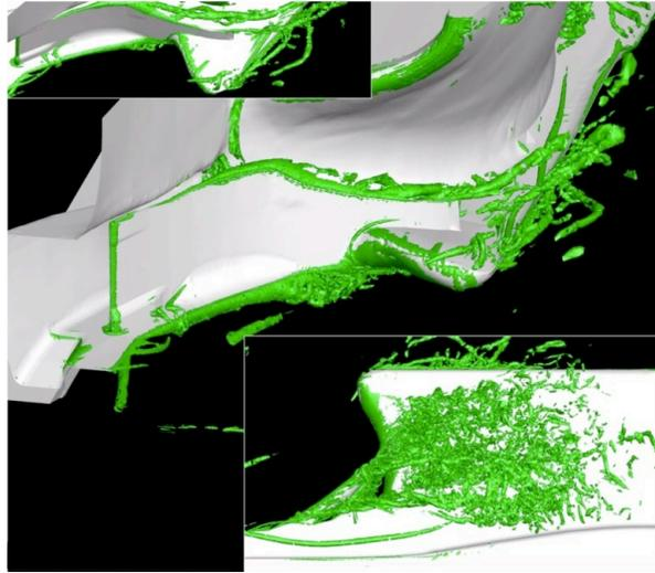
Figure 1: Vortical structures created by the side pod of a formula 1 car
