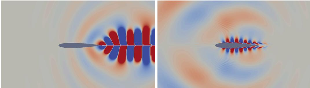
Linearised direct (left) and adjoint (right) simulations of the flow around an aerofoil at  $Re = 15000$  and  $M = 0.6$  at zero incidence.
