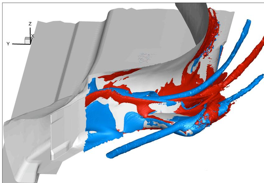
(a) 3d view of the sidepod system, counter-clockwise (blue) and clockwise vortices (red), isosurfaces of normalised helicity
