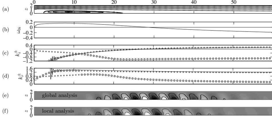
Figure 1: (a) base flow; (b) local absolute growth rate; (c) local spatial growth rate; (d) local wavenumber; (e) eigenfunction from global analysis; (f) eigenfunction from local analysis.
