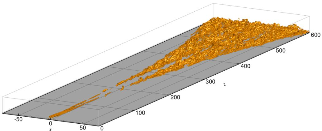
Figure 1: By-pass transition in a swept Hiemenz flow at  $Re = 300$  (isosurface of the  $\lambda_2$  vortex criterion with  $\lambda_2 = -0.001$ ).
