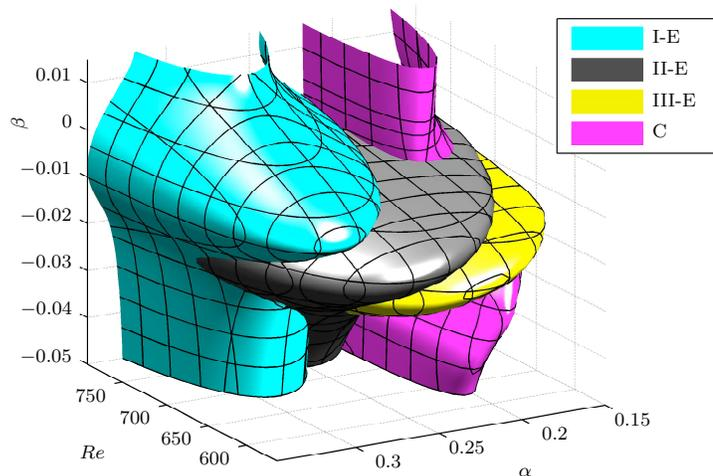
Isometric view of neutral surfaces of different modes for  $Ma = 0.01$ : (cyan) I-E, (gray) II-E, (yellow) III-E, (magenta) C
