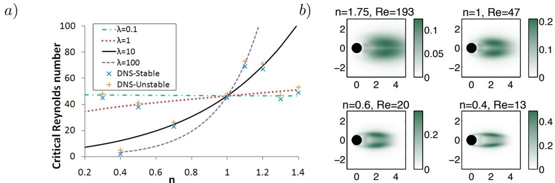
Figure 1: a) Neutral stability curve for the flow past a circular cylinder of a Carreau fluid in the Reynolds– $n$  plane for different values of the material time constant  $\lambda$ .  $n < 1$  indicate shear-thinning behavior whereas  $n > 1$  indicate a shear-thickening fluid. b) Wave-maker, the core of the instability, along the neutral curve for  $\lambda = 10$  and 4 values of the exponent  $n$ .
