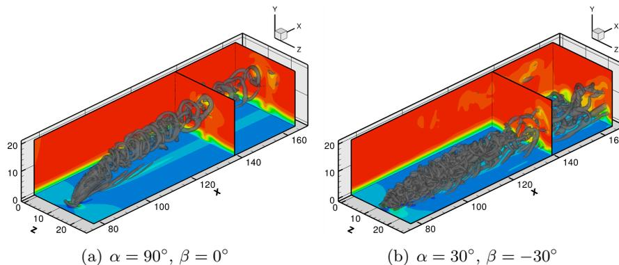
Vortex structures and  $u$ -velocity contours of Jet-in-Crossflow computations
