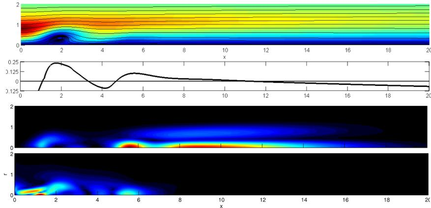
Figure 2: (a) base flow; (b) abs. growth rate; (c) wavemaker region (d) sensitivity to base flow modif.
