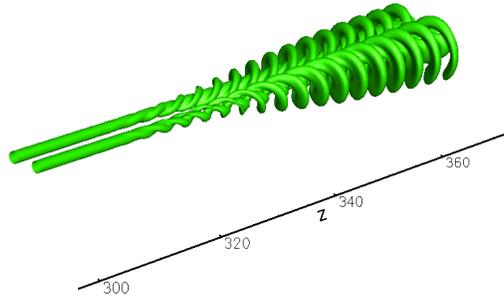
**Figure 1.** Iso-surface of axial velocity flow field ( $\bar{u} = U + \varepsilon u$ ) with  $\varepsilon = 10^{-4}/|u_0|$  in the range  $x \in [300, 370]$
