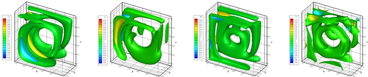
**Figure 1.** Amplitude functions corresponding to the leading eigenmode of the regularized lid-driven cavity flow at  $Re = 10^3$  with  $L_z = 2\pi/15$ . Left-to-right:  $\hat{u}(x, y, z)$ ,  $\hat{v}(x, y, z)$ ,  $\hat{w}(x, y, z)$ ,  $\hat{p}(x, y, z)$ .
