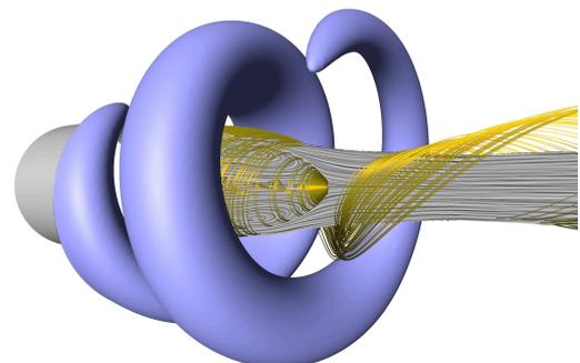
(b) Theoretically extracted coherent structure using linear stability analysis
