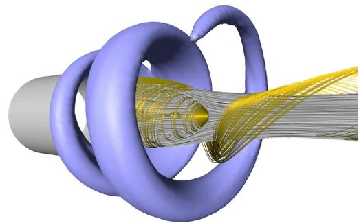
(a) Empirically extracted coherent structure using POD
