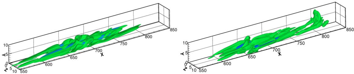
Figure 1: Snapshots of the streamwise component of the perturbation (blue) and of the Q-criterion (green) on the edge of chaos for a linear (a) and non-linear (b) initial perturbation.
