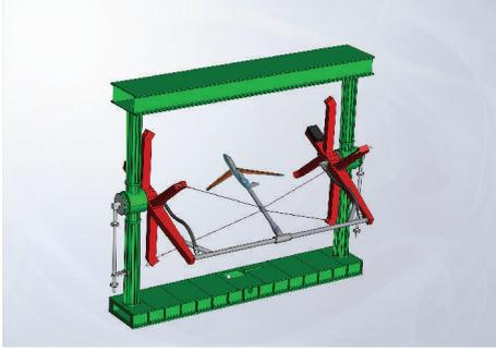
Figure 1: Schematic of wire assistant sting support system.
