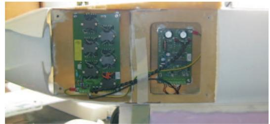
Figure 2: Minipuls 0.1 high voltage generator installed in fuselage.
