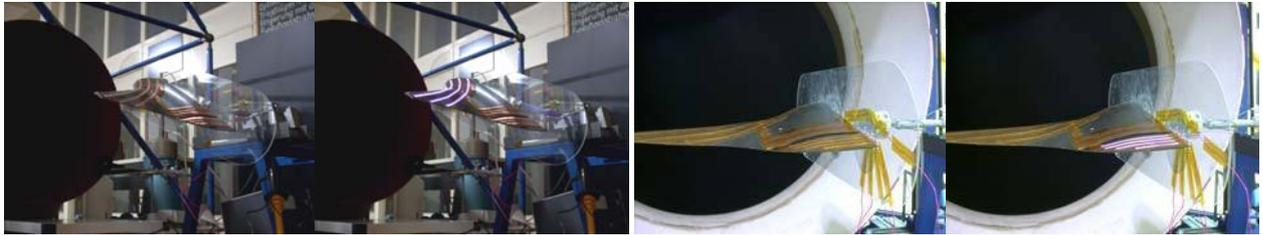
Figure 4a-4d. Four phase shifted plasma actuators on leading and trailing edge of a flying wing half-span model.
