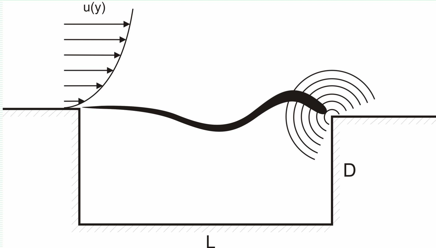
Numerical simulation of self-sustained oscillations
