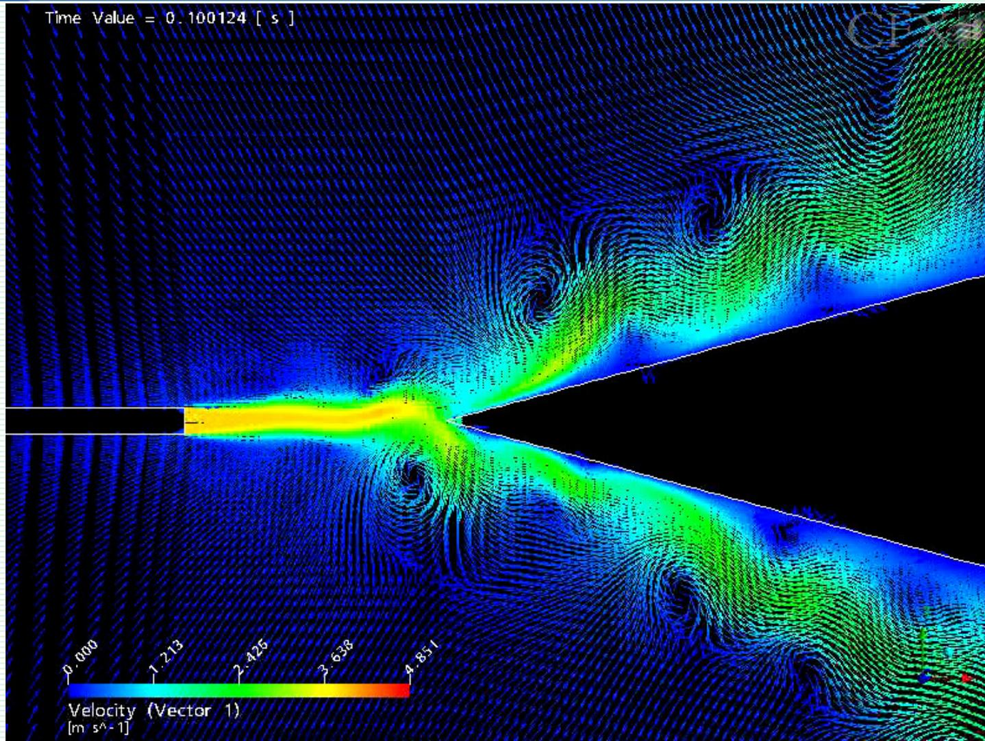
Numerical simulation of self-sustained oscillations
