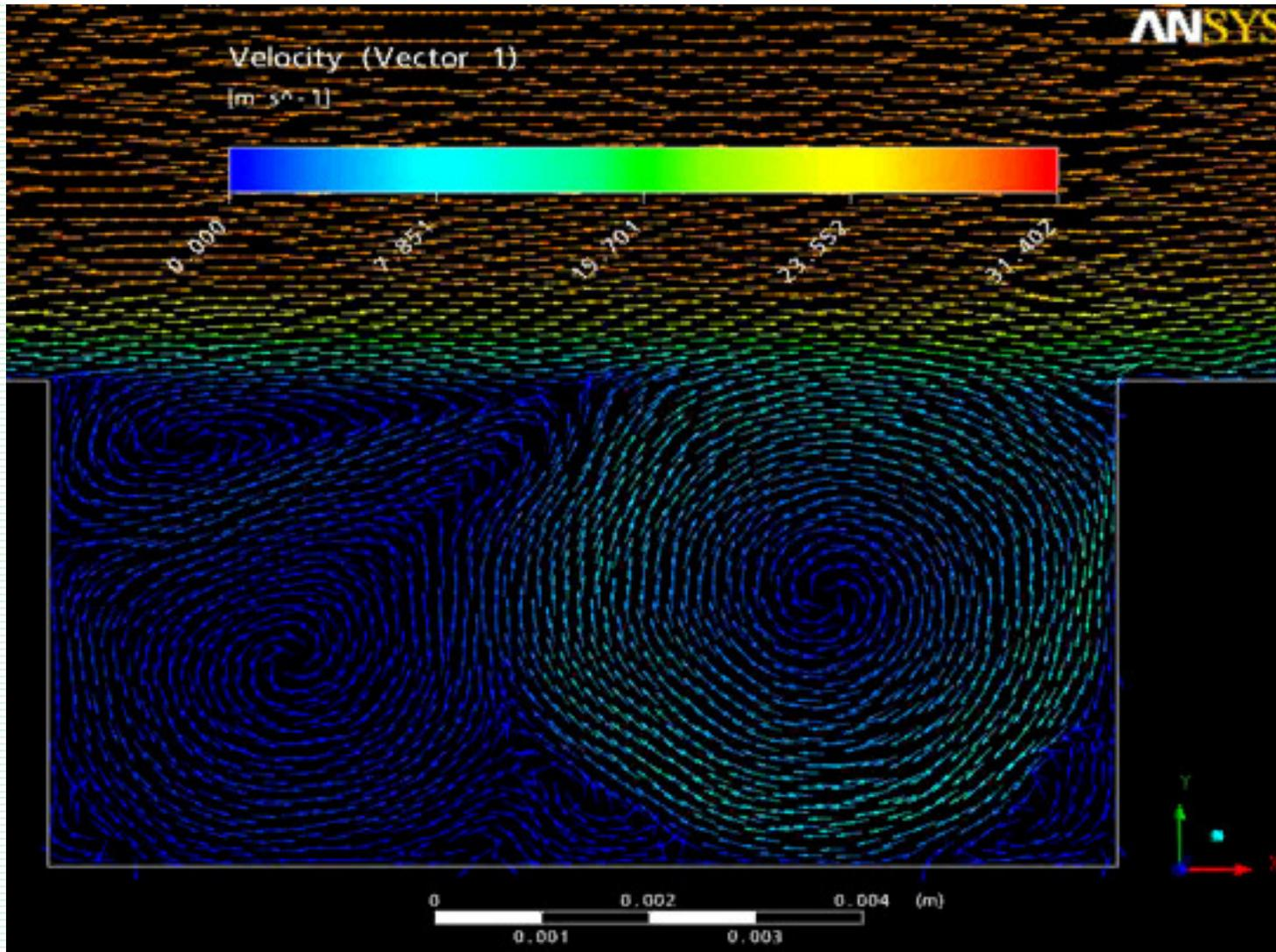
Numerical simulation of self-sustained oscillations
