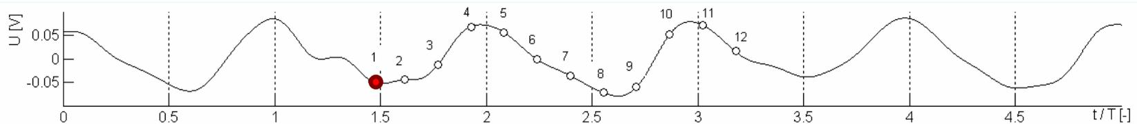
Numerical simulation of self-sustained oscillations
