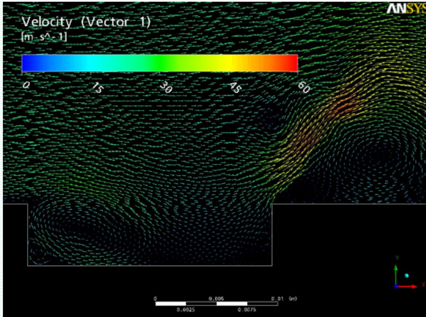
Numerical simulation of self-sustained oscillations
