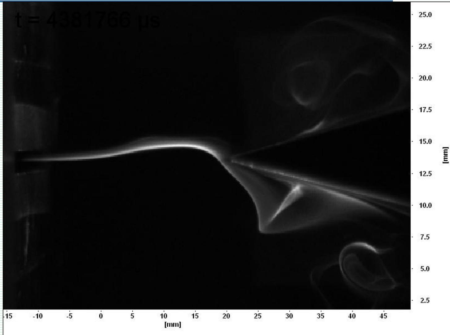
Numerical simulation of self-sustained oscillations
