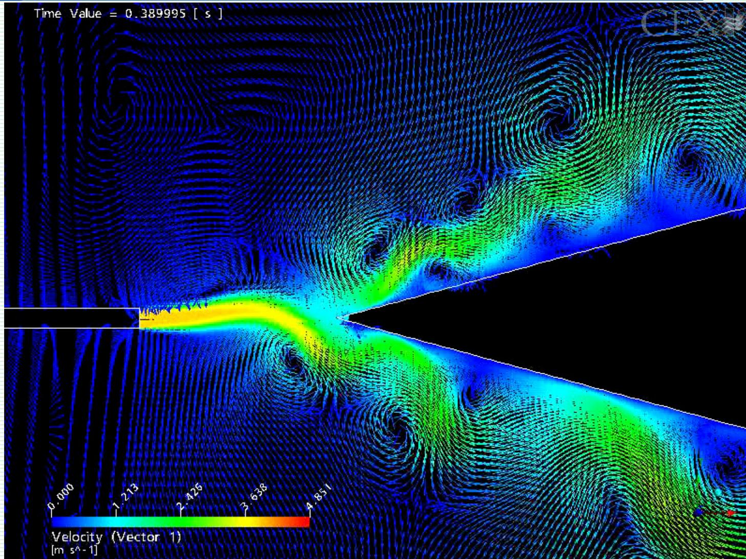
Numerical simulation of self-sustained oscillations
