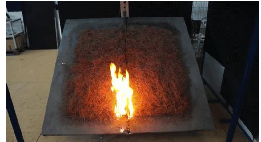
Temporal evolution of fire front developing at 30° slope angle (x64 time)
