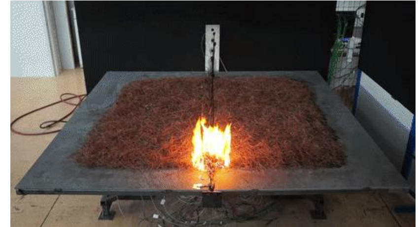
Temporal evolution of fire front developing at 0° slope angle (x64 time)
