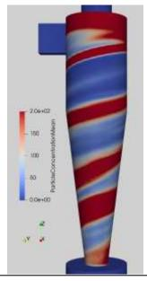
Euler/Lagrange results for particle separation in a 290mm gas Cyclone with rope formation, inlet velocity 10 m/s, mass loading 1.0, MPS-OvGU 2023)
