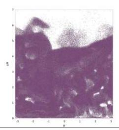
CFD/DEM simulation of the instantaneous particle distribution in a fluidised bed close to the wall; particle size 875 microns, solid density 740 kg/m³, fluidization velocity is 0.32m/s and the number of tracked particles is **9 631 313** representing a total mass of 2.5 kg (IMFT, Toulouse, 2024).
