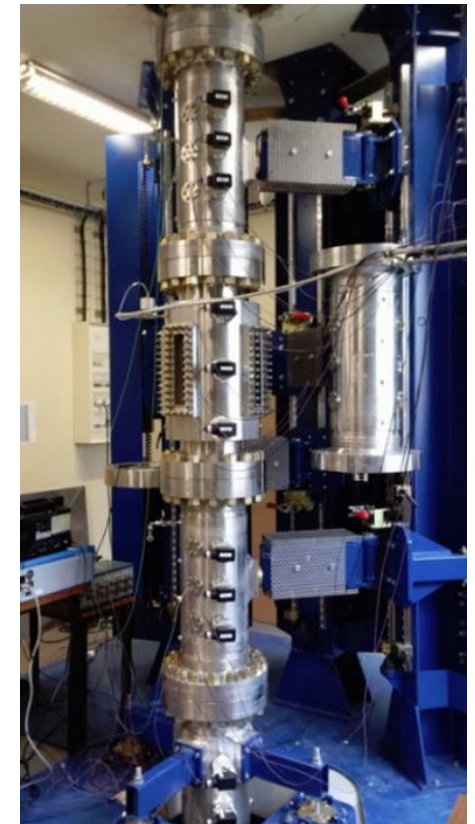
Photo of ENACCEF2 test rig [1] .
