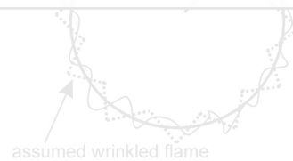
Schematic of a flame-surface-based phenomenological model for explosions [2] .
