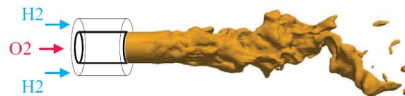
Figure 7: Density iso-surface  $\rho=30 \text{ kg/m}^3$
