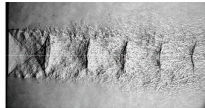
Figure 15: Schlieren visualization of an underexpanded jet (convergent nozzle,  $NPR = 2.5$ )
