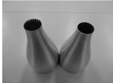
Figure 1: Photograph of the notched nozzle (left) and the baseline nozzle (right).
