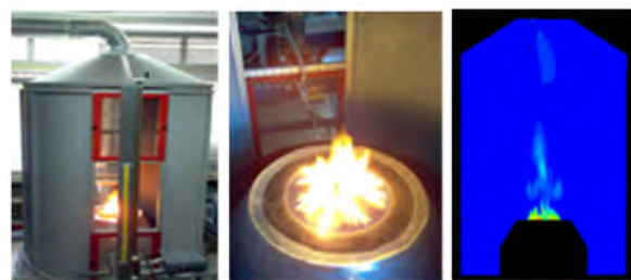
Figure 12: Axisymmetric fire plume experiment and LES simulations
