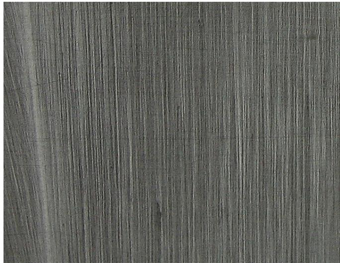
Figure 4: Suction Surface Flow Visualisation between 80% and 95% Axial Chord of NRC Turbine Blade at a Discharge Mach Number of 1.16
