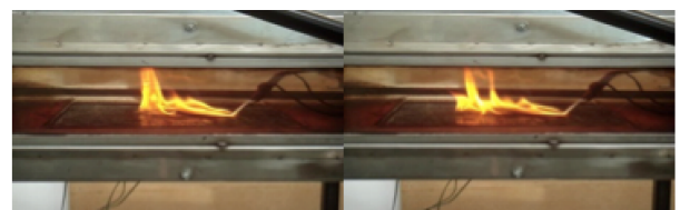
Figure 15: Fire spreading in Hidden Fire Apparatus
