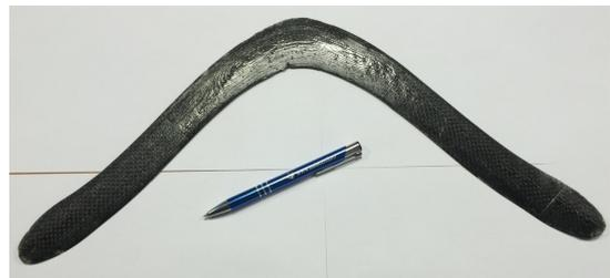
Figure 10: The boomerang prototype obtained using epoxy resin and carbon fibers on a 3D printed mould
