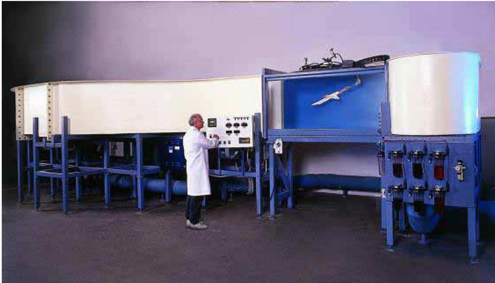
The Rolling Hills Research Corporation Flow Visualization Water Tunnel
