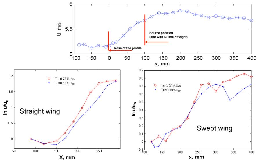
Downstream behavior of the boundary layer disturbances amplitude at the low and hi free stream turbulence level
