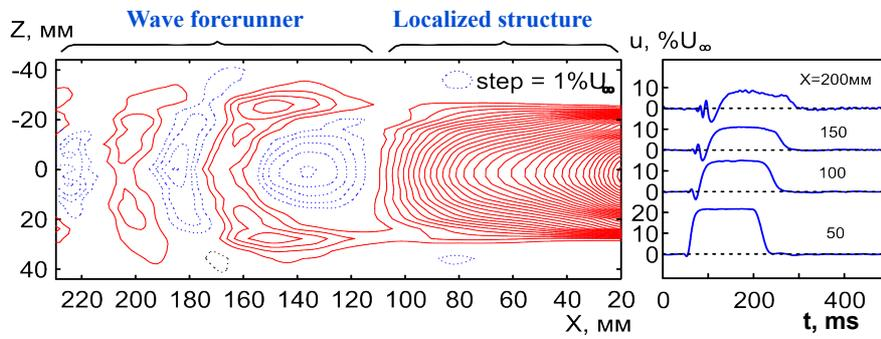
Hot-wire anemometry visualization of the localized structure and the wave forerunner near the leading front of the streak. The localized structure was generated by suction through the spanwise slot.
