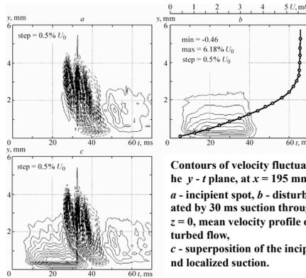
Contours of velocity fluctuations  $u'$  in the  $y-t$  plane, at  $x = 195$  mm,  $z = 0$ .
