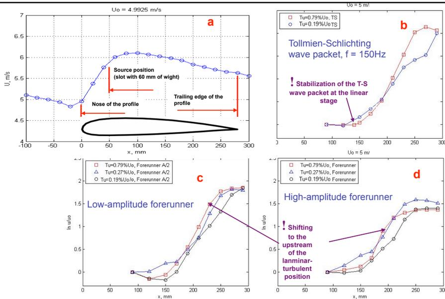
(a)-mean velocity  $U$  distribution outside the boundary layer; (b,c,d)-distribution of the velocity fluctuations ( $u_{y_{max}}$ ) at the maximum level of fluctuations in  $Y$  direction along the wing chord.
