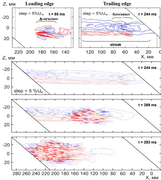
Origination of the Δ-structure from the wave forerunner at the leading edge of the localized disturbance.
