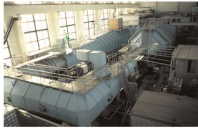
Low-turbulence wind tunnel T-324
