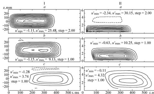
Contours of velocity fluctuations  $u'$  in the  $z$ - $t$  (I) and  $y$ - $t$  (II) planes, large amplitudes. The source of disturbances is a transverse slot at  $x = 95$  mm. The disturbance is generated by suction during 300 ms. I:  $x = 100$  (a), 200 (b), 500 mm (c); II: a-  $x = 100$  mm,  $\delta = 3$  mm; b-  $x = 200$  mm,  $\delta = 4$  mm; c-  $x = 500$  mm,  $\delta = 6$  mm.
