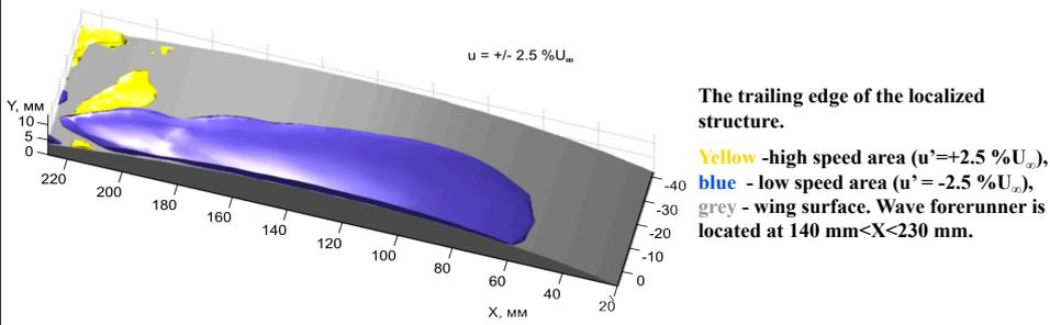
**Contours of the high-frequency components of velocity fluctuations**
