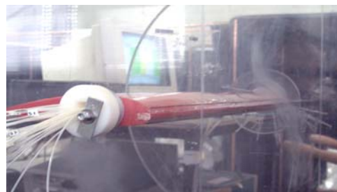
Pitot/HWA flow measurement around NACA0012 airfoil
