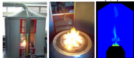
Axisymmetric fire plume experiment and LES simulations
